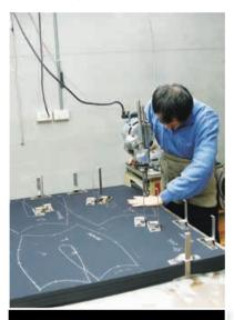
The cutting machine slices through the neoprene sheets.
