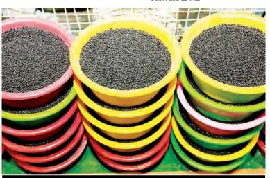
These are the pellets used as dying material in the foaming procedure.
