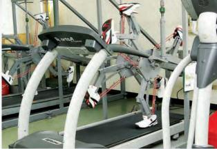
Sports Art's facility in Tainan has an extensive testing facility, to check the functionality and the durability of the products. Tests on strength machines are set at one million lifts and these shoes will run for many miles.
