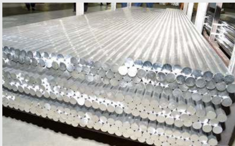
Extruded aluminum bars ready to be made into headset and bottom bracket shells and other parts.
