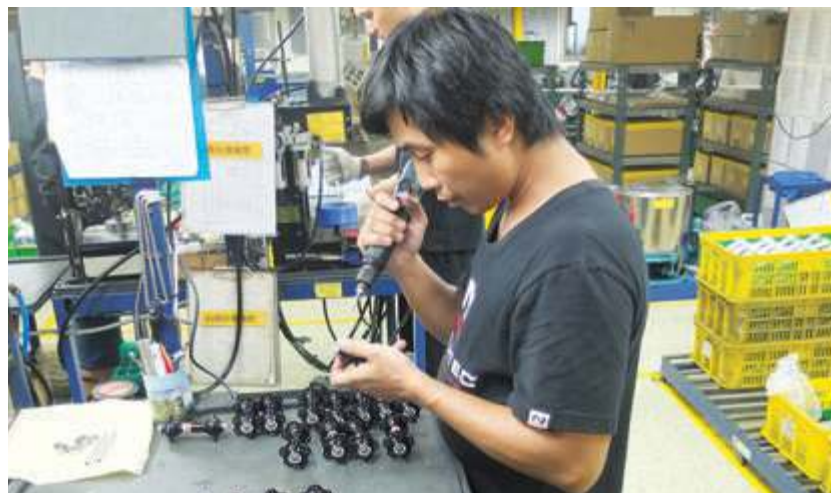
Experienced workers assemble Novatec hubs.
